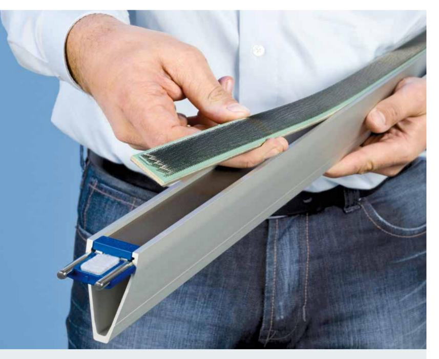
The clothing strip on the MAGNOTOP flats system is attached precisely and securely to the flat bar by ultra-strong magnets.
