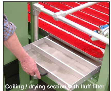
Coiling / drying section with fluff filter
