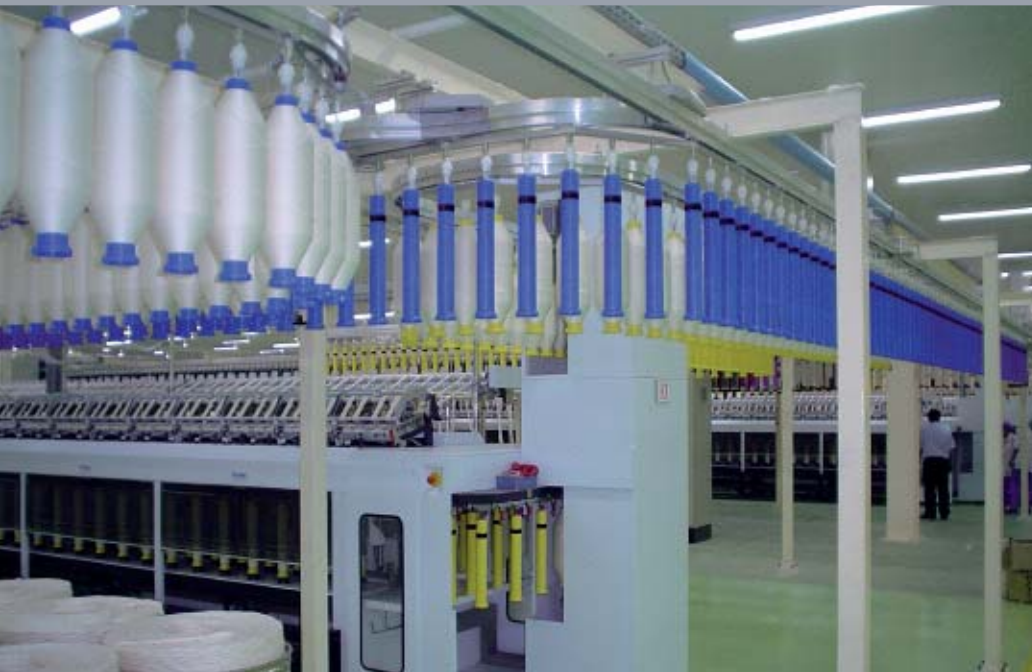
Textra – Flyerspulen-Transportsystem Textra – roving bobbin transport system
