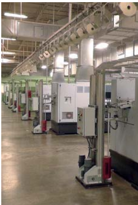
Kreuzspulenlifter und Textra-Spulentransportsystem an OE-Spinnmaschinen Package lifter and Textra-package transport system at OE-spinning frames
