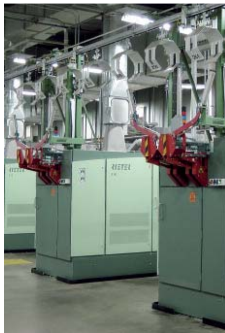
Kreuzspulenlifter und Textra-Spulentransportsystem an OE-Spinnmaschinen Package lifter and Textra-package transport system at OE-spinning frames
