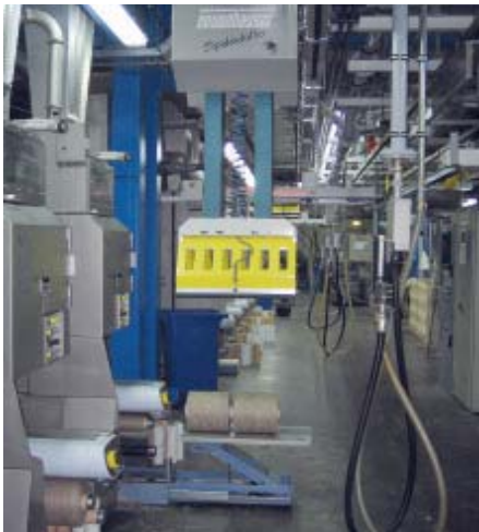
Spider Doffer am BCF-Spulenwickler Spiderdoffer at BCF yarn winder
