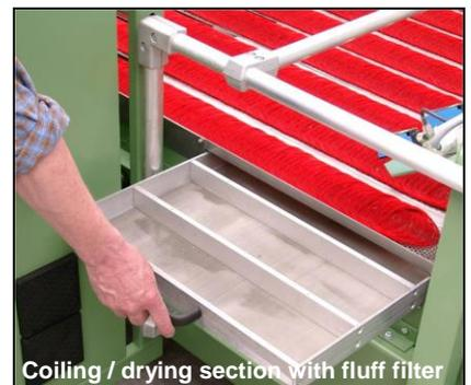
Coiling / drying section with fluff filter
