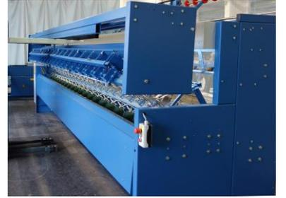
Easy removal of band magazine unit (with fork lift or crane)
